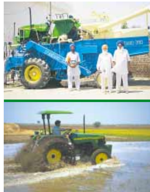
Above: Tractors fitted with cage wheels are used to prepare paddy fields for rice planting.
