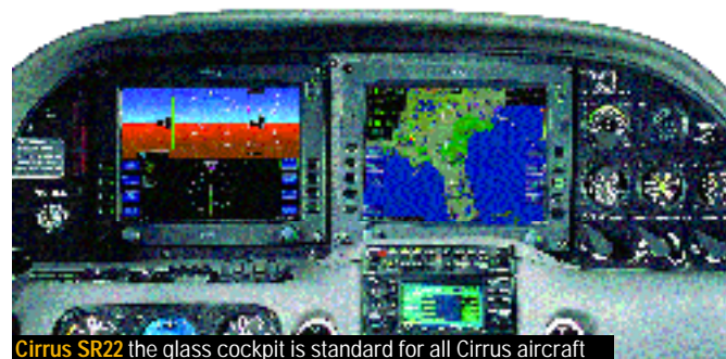
Cirrus SR22 the glass cockpit is standard for all Cirrus aircraft
