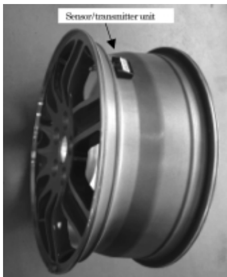
Fig. 2 Sensor/transmitter unit on wheel
