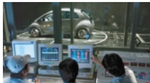
Fig. 7 Testing of full-size vehicle in wind tunnel
