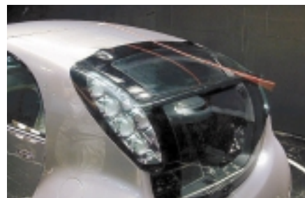
Fig. 8 Airflow over roof spoiler
