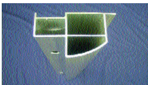
Fig. 3 Cross-sectional view of extrusion forming dash cross member lower
