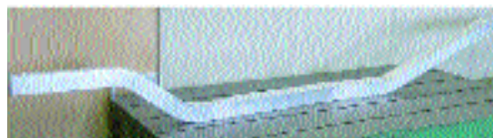
Fig. 4 One-piece side member
