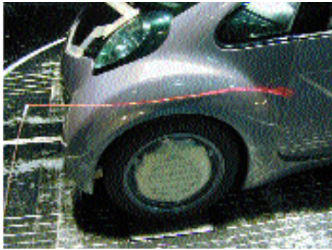
Fig. 23 Visualization of airflow around front fender
