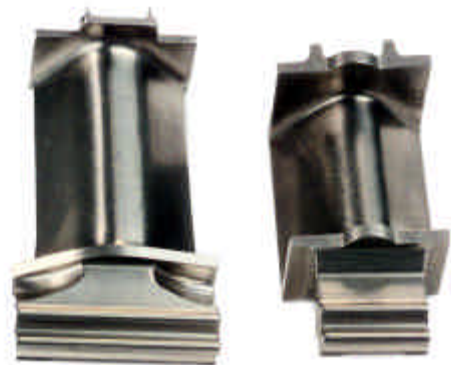
Figure 7: First-stage blade of the Fuel TP turbine (left) and the Vulcain 2 first-stage blade of the Oxygen TP turbine.
