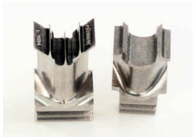
Figure 7: First-stage blade of the Fuel TP turbine (left) and the Vulcain 2 first-stage blade of the Oxygen TP turbine.
