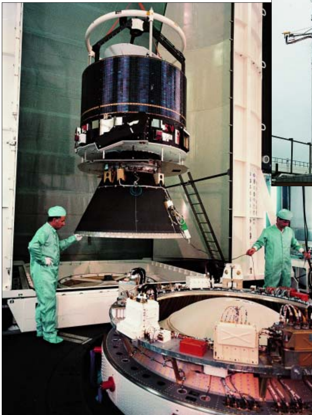
Installation of Giotto on its Ariane launcher at Kourou. The dome cover of the third stage liquid hydrogen tank can be seen protruding through the centre of the Vehicle Equipment Bay. (CSG/CNES/Arianespace)
