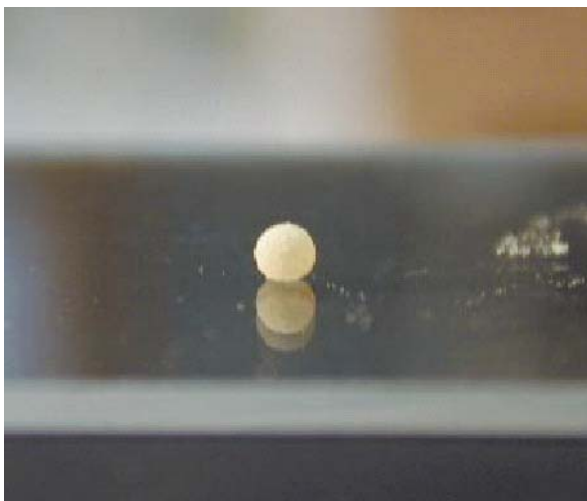
Figure 20: A liquid marble: water coated with silane-treated lycopodium grains of typical size 20nm). (From: Aussillous 26 )
