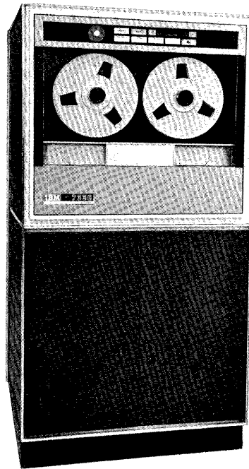
Figure 90. IBM 7330 Magnetic Tape Unit
