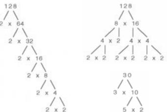
**Figure 1.** The FFT applies when N is a power of 2, with the classic decomposition shown in Figure 1a (left) and an alternative in Figure 1b (top right). When N is no longer restricted to powers of 2, the best decomposition might look like that shown in Figure 1c (bottom right).
