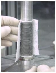
thermal battery's desirable characteristics. The material is completely inert and nonconductive until the battery is activated at which time it becomes molten and highly conductive. This allows the cathode to interact with the anode.
