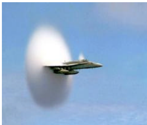
Figure 1. Condensation cloud (from http://www.chinfo.navy.mil/navpalib/images/hornetsb.jpg . U.S. Navy photo by Ensign John Gay. [990707-N-6483G-001] July 7, 1999)
