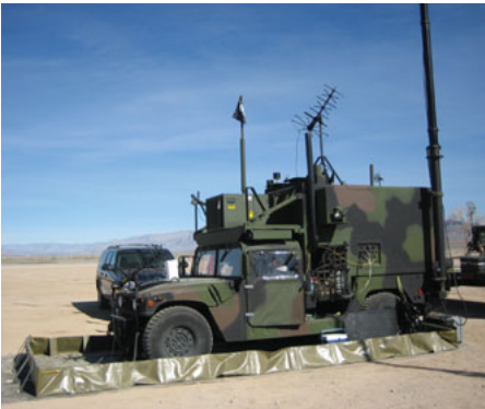
RAIDER provides a connection point for BACN to the terrestrial GIG and supports ground forces on the Tonopah Range
