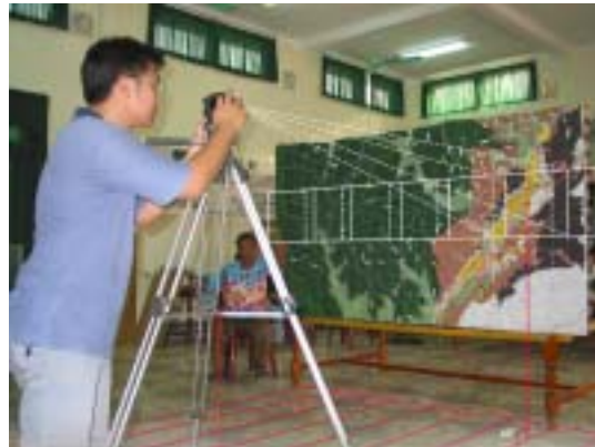
Figure 5. Parallel Camera Movement shooting to capture digital high resolution images of the landscape
