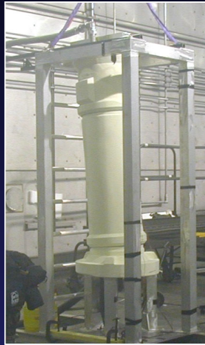
Lower Feedline Bellows During Baseline Test at Eglin AFB
