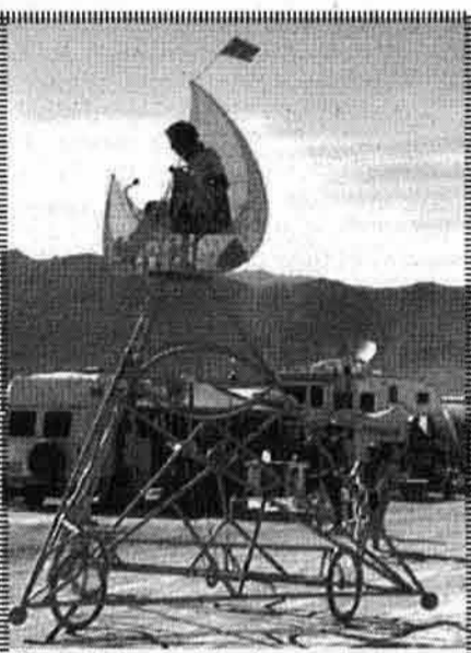
Three-wheel moon bike. Looooong chain goes to rear axel, looon front fork steers
