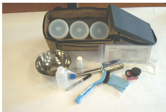
Figure 5. Deployment Soil Sampling Kit
