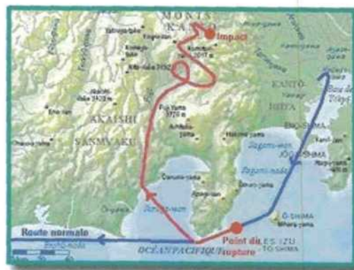
Figure 5. Flight path following explosive decompression depicted in red.
