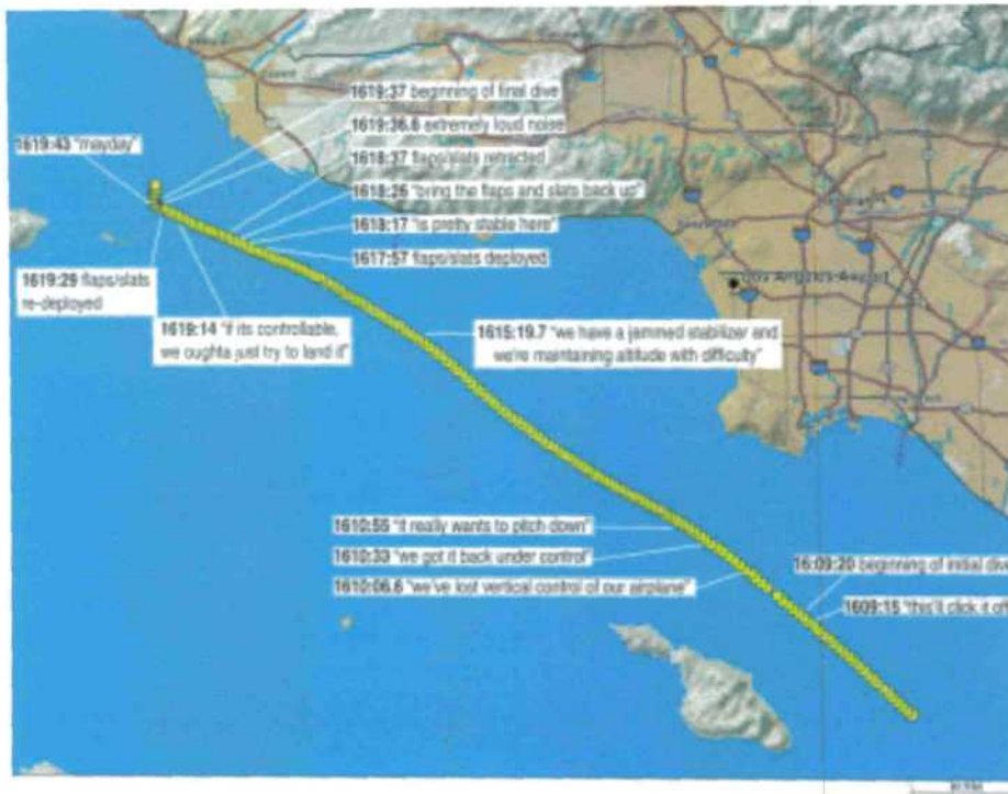
Figure 7. The flight path of Alaska Airlines Flight 261, starting about 1609 (about the time of the initial dive) and ending about 1620 (about the time of the second and final dive).
