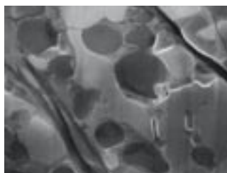
Nova FIB section of Sun Screen cream imaged at 10.0 kV with the TLD-SE detector
