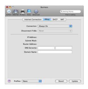
• Choose Always On, Automatic, or Manual, depending on how you want to control when your wireless device is connected to the Internet.
