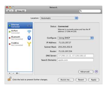
c If you selected "Distribute a range of IP addresses" when you set up the wireless device's network, you can provide Internet access to client computers using Ethernet by setting the client IP addresses manually. Select Ethernet in the network connection services list, and then choose Manually from the Configure pop-up menu.
