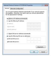
• If you chose "Distribute a range of IP addresses" when you set up the wireless device's network, you can provide Internet access to client computers by setting the client IP addresses manually. Select "Use the following IP address."
