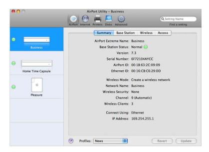
You can also double-click the name of the wireless device to open its configuration in a separate window. When you open the manual setup window, the Summary pane is displayed. The summary pane provides information and status about your wireless device and network.
