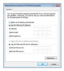
When you configure clients manually for a wireless device that provides NAT service, use IP addresses in the range 10.0.1.2 to 10.0.1.200, 172.16.1.2 to 172.16.1.200, or 192.168.1.2 to 192.168.1.200.
