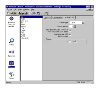
• If the source is connected to another Meridian unit, set Comms type to 1C for a Meridian CD player, 2C for a Meridian FM tuner, and 3C for a Meridian DVD player. Otherwise set it to none.
