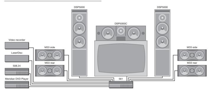
The 561 Digital Surround Controller can be used with two Meridian DSP5000 Digital Loudspeakers, and a DSP5000C Digital Centre Loudspeaker, to provide audiophile-quality sound. A further two or four M33 Active Analogue Loudspeakers can be added as side or rear loudspeakers to give extremely convincing multi-channel reproduction from music and film sources.
