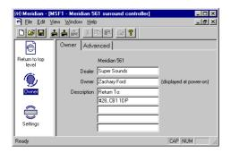
The **Owner** text will be displayed when you turn the 561 on. The **Dealer** and **Description** text are displayed after the product version and serial numbers if you hold down the front-panel **Display** key in standby.
