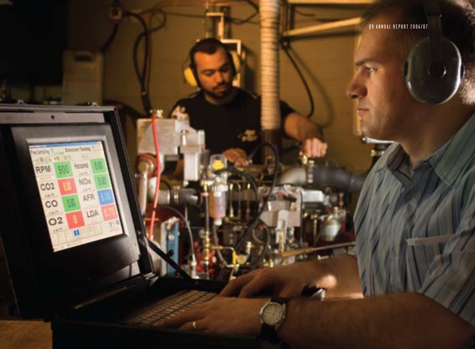
Rail CRC Researcher, Dr Damon Honnery, works in the Monash Diesel Engine Test Facility on Project 55 'The Assessment of the effect of diesel fuel additives on locomotive performance and operation'.
