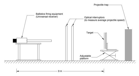
Figure C-1. Schematic of the ballistic research test facility.
