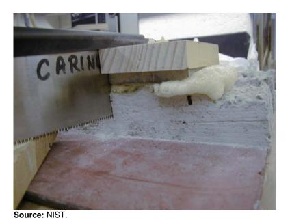
Figure 7–12. Preparing the SFRM specimen for adhesion/cohesion test.
