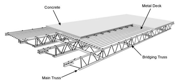
Figure 3–2. Schematic of composite floor truss system.
