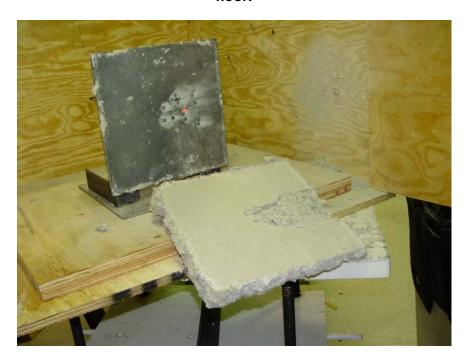
Figure C-6. Photograph showing damage to the SFRM after a ballistic impact at 40 degree. The SFRM layer completely separated from the steel plate.
