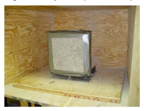
Figure C-8. Photograph showing the edges of the SFRM duct taped to the steel plate before the ballistic tests at 0 degree.
