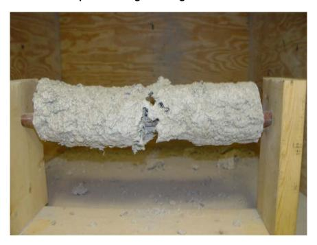
Figure C-10. Photograph showing damage to the SFRM on a primed steel bar (BAR02) after a ballistic impact at 0 degree using the small universal receiver.
