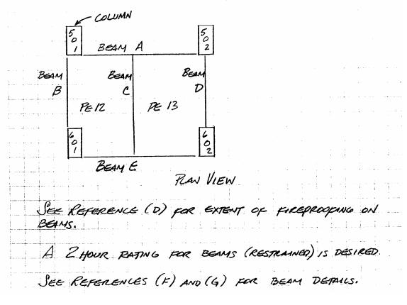
Figure A–47 (Contd.). Excerpts from 1992 report on thermal insulation thickness for repair of missing insulation (240-LERA).
