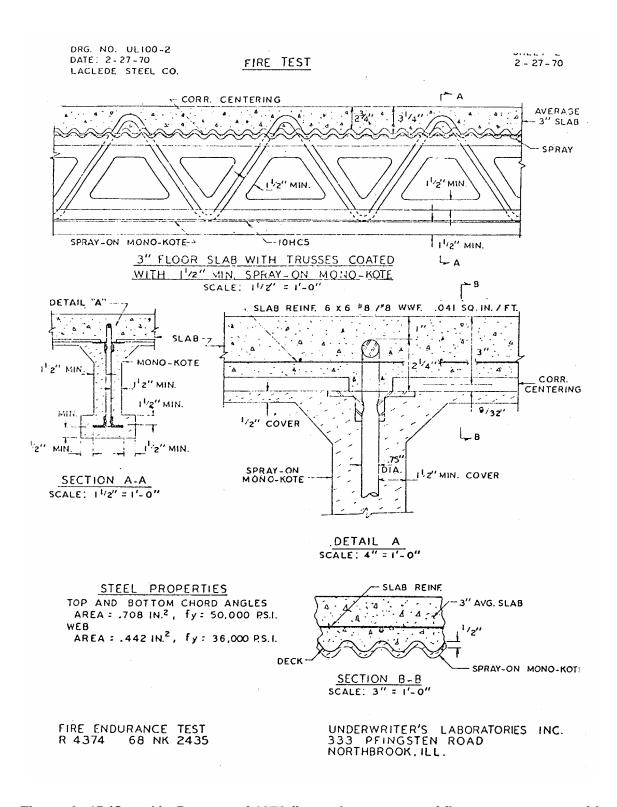
Figure A-45 (Contd.). Reports of 1970 fire endurance test of floor truss system with sprayed thermal insulation (3-P).
