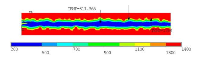
Figure 5–2. Temperature distribution after 1 h of exposure to gas temperature of  $1,100~^{\circ}$ C (1,373 K).
