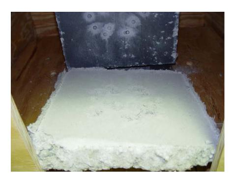
Figure C-4. Photograph showing damage to the SFRM after a ballistic impact at 0 degree.
