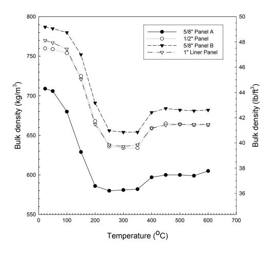
Figure 6–13. Bulk densities of the four gypsum materials as a function of temperature.
