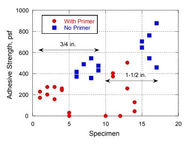
Figure 7–23. Adhesive strength of BLAZE-SHIELD DC/F specimens for primed and unprimed steel plates.
