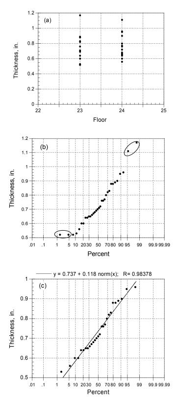
Figure 4–1. (a) Dotplot of average thickness from floor trusses for floors 23 and 24, (b) normal probability plot of all average thickness values, and (c) normal probability plot of average thickness with four values (six points) excluded.
