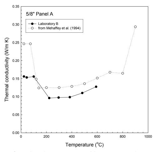
Figure 6–10. Comparison of the thermal conductivity measurements from Laboratory B with the data from Mehaffey et al. (1994) for 5/8 in. thick gypsum panel A.
