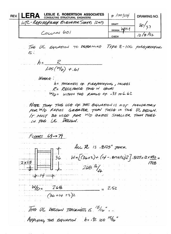
Figure A–47 (Contd.). Excerpts from 1992 report on thermal insulation thickness for repair of missing insulation (240-LERA).
