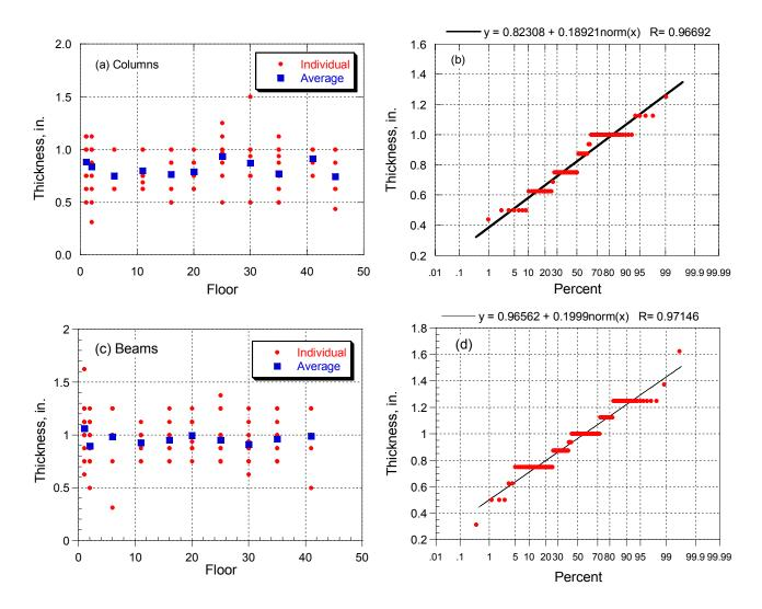
Figure 4–6. Thickness of re-applied SFRM in elevator shaft 10/11 of WTC 1: (a) Individual and average thickness for core columns, (b) normal probability plot of individual measurements on columns, (c) individual and average thickness for core beams, and (d) normal probability plot of individual measurements on beams (data provided by PANYNJ).
