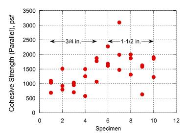
Figure 7–19. In-plane cohesive strength for BLAZE-SHIELD DC/F specimens.
