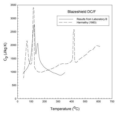
Figure 6–7. Comparison of specific heat capacity measurements for BLAZE-SHIELD DC/F from Laboratory B with the results from Harmathy (1983).
