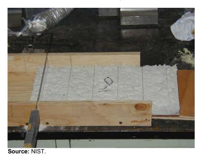
Figure 7–9. Cutting the SFRM layer into five strips.
