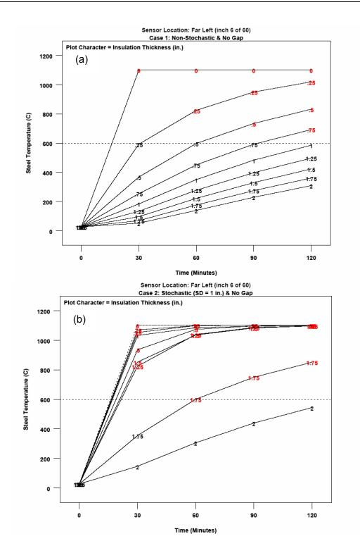
Figure 5–3. Variation of steel temperature (at a point 6 in. from end of plate) with time for different average thicknesses of fire-resistive material (shown as numbers on the curves): (a) uniform thickness, and (b) variable thickness with standard deviation = 1 in.
