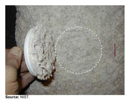
Figure 7–2. Cohesive failure of SFRM using ASTM E 736 test (dashed circle is approximate location of cap before being pulled off.
