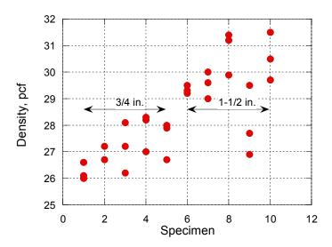
Figure 7–17. Density of BLAZE-SHIELD DC/F specimens.
