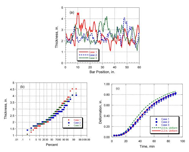
Figure 5–8. (a) Randomly generated thickness profiles with average thickness of 2.5 in. and standard deviation of 0.6 in., (b) normal probability plots of thickness values, and (c) deformation of 1 in. bar compared with deformation for uniform thickness of thermal insulation.
