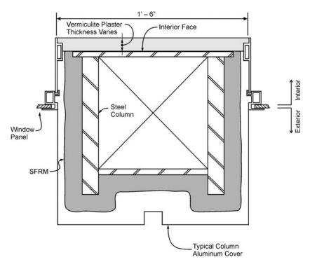
Figure 3–4. Thermal insulation for perimeter columns.
