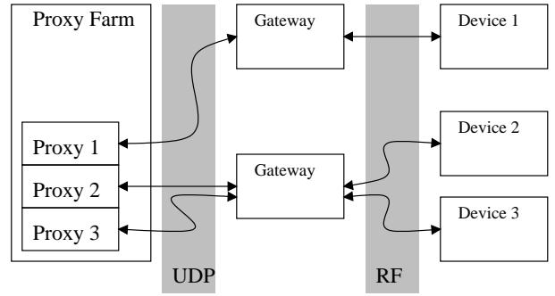
Figure 3: Device-to-Proxy Communication overview
