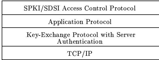
**Figure 5: Example Layering of Protocols**
