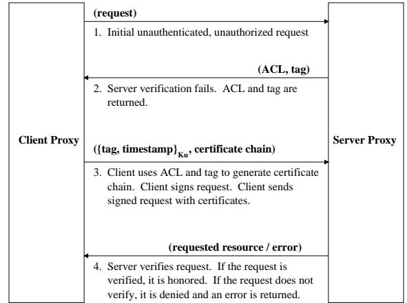
**Figure 4: SPKI/SDSI Proxy to Proxy Access Control Protocol**
