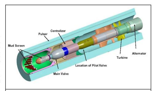
Schematic of the bi-directional power and communications module MWD component. The surface control system communicates via mudpulse signals. The turbine/alternator provides power to other MWD components in the BHA.
