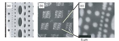
**Figure 8.** Patterning of NV centres in type Ib diamond via implantation through a mask. (a) The quantifoil carbon grid used to mask the sample during ion implantation. The grid was coated with Au to increase the stopping power. Confocal luminescence imaging ((b) and (c)) shows that the mask pattern is faithfully transferred to the sample.
