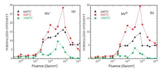
**Figure 7.** The intensity of (a) the NV<sup>-</sup> (637 nm) and (b) the NV<sup>0</sup> (575 nm) ZPL normalized to the intensity of the first order Raman mode (at 1332 cm<sup>-1</sup>) as a function of Ga ion fluence. The Ga ion energy was 30 keV. Data for post-implantation annealing at 600, 800, and 1000 °C are shown. The PL was excited by 514 nm excitation and the spectra collected at 77 K.
