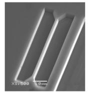
Figure 4. SEM image of a waveguide structure created in single crystal diamond with the FIBassisted lift-off technique; the structure has a cross section of  $3.5 \times 2 \ \mu m^2$ , while the 500 nm undercut is visible.
