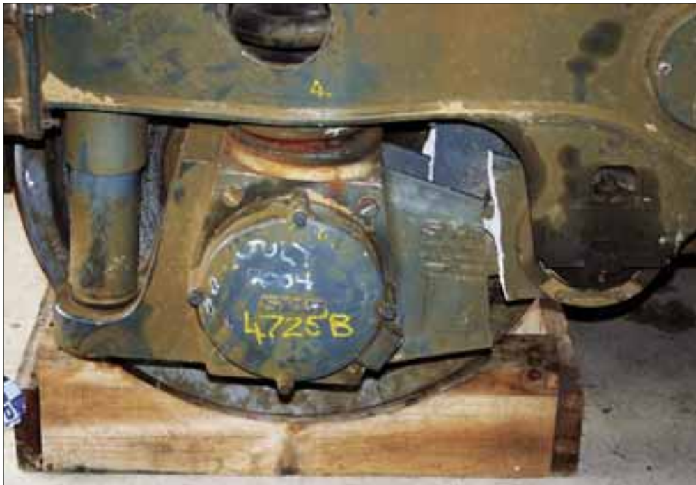
FIGURE 13: Fractured trailing arm – leading axle, left side
