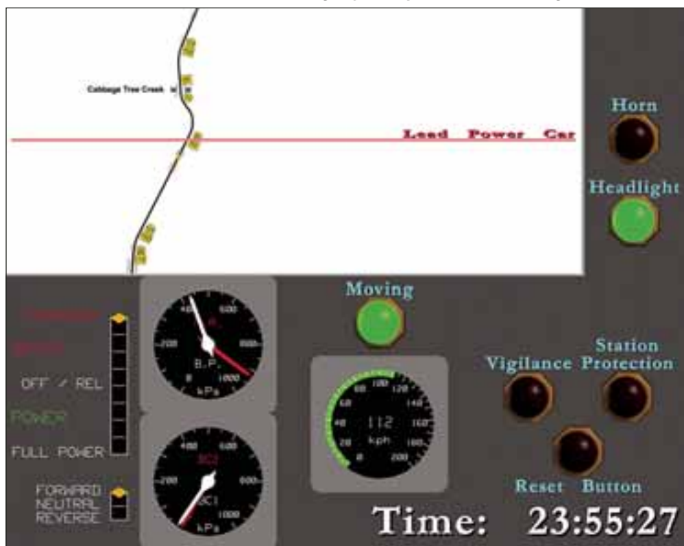
FIGURE 7: Power/Brake Controller in full emergency brake position, train travelling at 112 km/h
