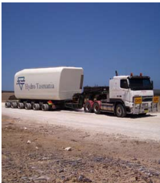
Wind turbine nacelle arrival at Cathedral Rocks Wind Farm
