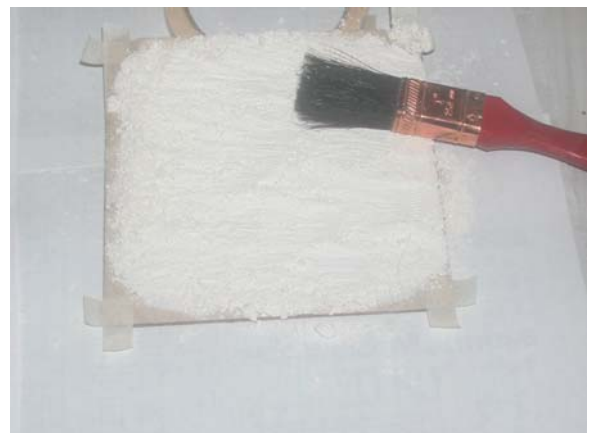
Figure 4. Diatomaceous earth pressed into glue with a clean brush.
