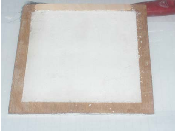
Figure 5. Finished device with masking tape removed and surplus diatomaceous earth brushed off.
