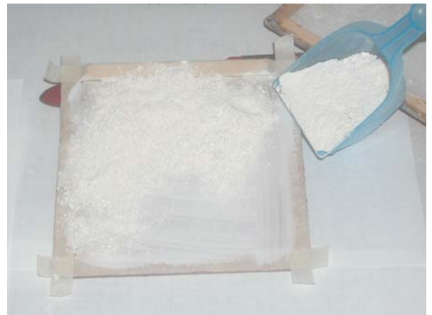
Figure 3. Diatomaceous earth applied as a thick coat
