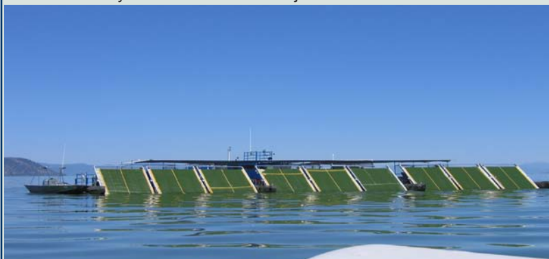
Self propelled floating platform for harvesting Aphanizomenon flos-aquae on Upper Klamath Lake. Note shuttle craft (left) for quickly moving freshly harvested algae to the processing facility. Source: Simplexity
