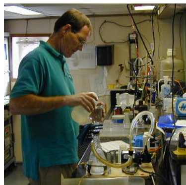
Filtering for microcystin analysis in Lake Erie. Photo: Steve Wilhelm, University of Tennessee
