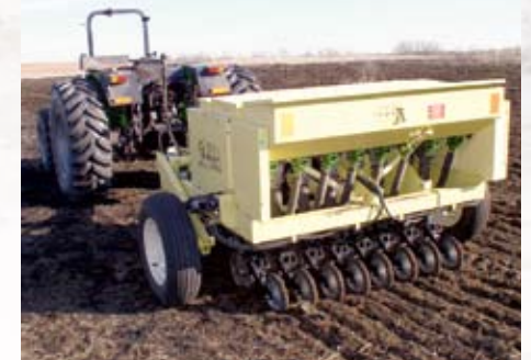
A grass drill has depth bands to ensure that grass seed is placed at the correct depth.
