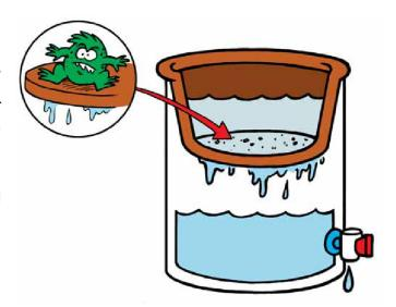
The filter element is an open-top clay cylinder. The filter is sometimes coated with colloidal silver, which helps to reduce the number of microorganisms in the water. The clay cylinder is placed in a plastic or ceramic receptacle with a lid and faucet. Pathogens and suspended material are trapped on the ceramic material as water is poured through the filter. If properly constructed and operated, a ceramic filter can be very effective in producing good quality water.
