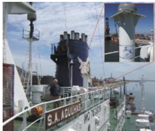
Fig 9. GPS Antenna on board the SA Agulhas for making ionospheric measurements in the South Atlantic Ocean during IPY/IHY.
