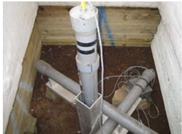
Fig. 2. The pulsation magnetometer operating at EFO (Ethio-Finno Observatory) at the top of Entoto Mountain in Ethiopia.
