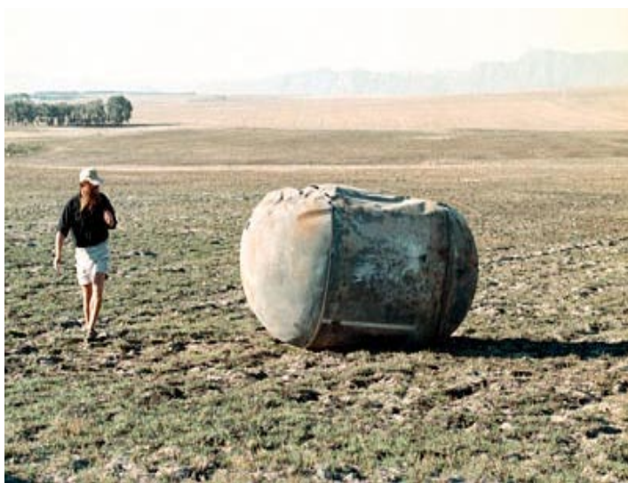
Fig. 3: A propellant tank from the second stage of a Delta II rocket, found on the farm Buurmanskraal, near Cape Town. Photograph by courtesy of Die Burger.
