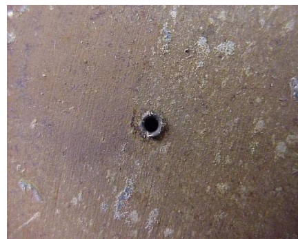
Fig. 4: This close-up of the propellant tank in Fig. 3 shows an impact site from a micro-meteorite. The crater is 2 mm across.
