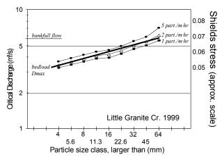
Fig. 9: Critical Discharge for Initial Motion: Largest Grain and Small Transport Rate Method.
