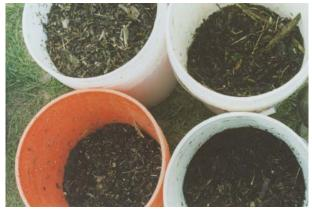
Fig. 5: Large Amounts of Organic Material may be Collected in the Bedload Traps.
