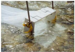
Fig. 2: Detail of Bedload Trap with Ground Plate.
