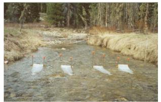
Fig. 3: Four Bedload Traps Installed at Little Granite Cr. at Low Flow (2002).
