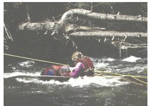
Fig. 4: Emptying Bedload Traps at Above Bankfull Flow at Cherry Cr., 1999.
