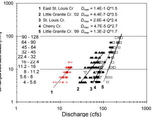
Fig. 7: Bedload Rating Curves from Bedload Trap Samples in Five Streams.
