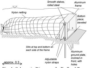
Fig. 1: Schematic Diagram of a Bedload Trap.
