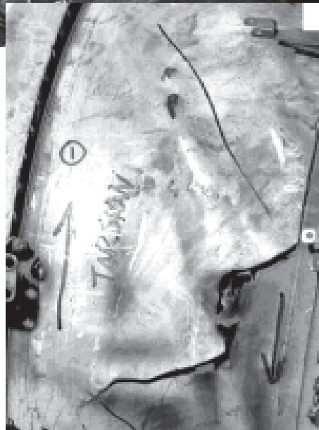
Figure 4. Buckled strut in turbine support.
