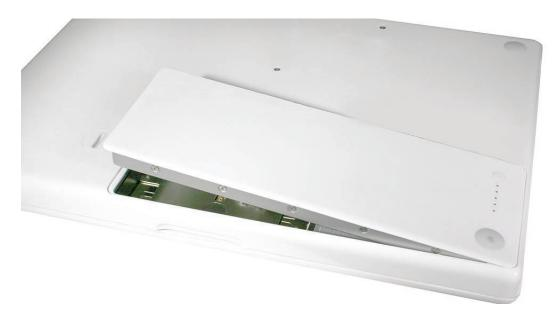
8. Touch a metal surface inside the battery bay to discharge any static electricity. Important: Always discharge static before you touch any parts or install any components inside the computer. To avoid generating static electricity, do not walk around the room until you have finished working and closed the computer.
