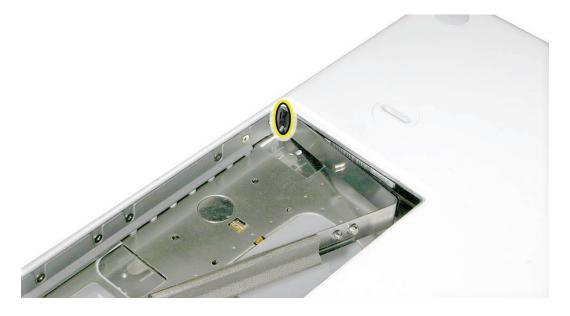
3. Use a plastic card, if necessary, to tuck in the EMI gaskets located on the RAM door so they do not protrude from the edge of the battery bay. Make sure the three screws align with the holes in the bottom case before tightening them.
