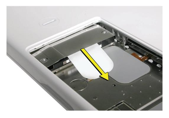
6. Hold the drive only by the sides when removing and replacing it.
