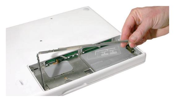
3. Important: Remember to replace the RAM door after you have finished working inside your computer. The computer will not function properly if the RAM door is not replaced.
