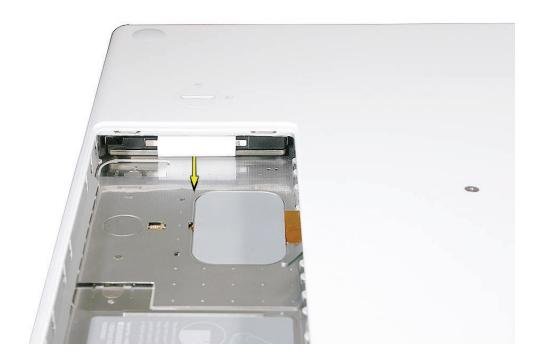
5. Pull the tab straight out to slide the drive out from the recessed rubber rails in the battery bay.
