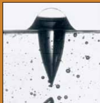
◀◀◀ Bubble reaching the free surface of a non-newtonian fluid. The peculiar fluid properties are responsible for the elongated bubble shape and the cusp formation at its tail
