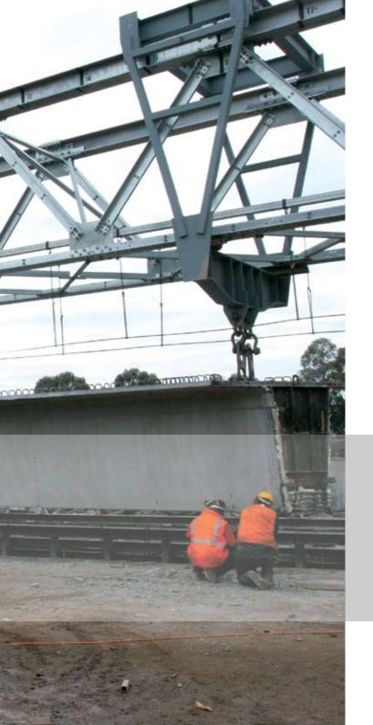
Our precast yard features two stressing beds, a precast bed and a pre-stress plant mould bed, to produce up to 700 tonnes of precast product per week. It also has one of Victoria's largest storage facilities for finished precast products.
