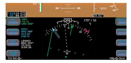
The wind vector on the HSI is very useful in any phase of flight where winds aloft should be taken into account. A combination of the wind vector and projected track line can be used to your advantage in navigation tasks. A very useful technique is to align the projected track line with the desired course. This will take the guess work out of determining proper crab angles for wind corrections.
