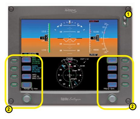
**1. Brightness Control (BRT/DIM)-** Controls display brightness. Power-on default is 75% brightness.
