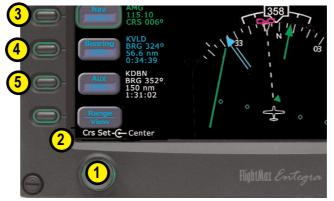
**1. Left Knob-** The function of the left knob changes based on which button on the left side is selected (indicated by green high-lighted ring around the button label). The symbol describes the rotary action of the knob. The symbol describes the push action of the knob.
