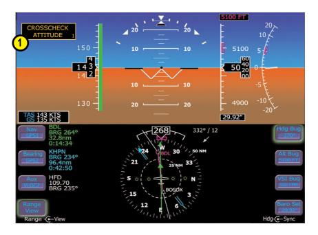
The *Entegra* PFD comes equipped with a self-check monitor. When the self-check monitor detects a condition that doesn't warrant removal of data, a directive warning message is displayed to the pilot to "CROSSCHECK ATTITUDE."
