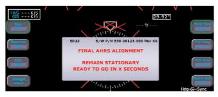
In the event that the AHRS is unable to complete its alignment, the following display is presented. If this occurs, wait approximately an extra two minutes in this state. If the system picks back up on the alignment, a nominal PFD will result. If the display does not clear itself, contact a service center and provide the displayed error code.
