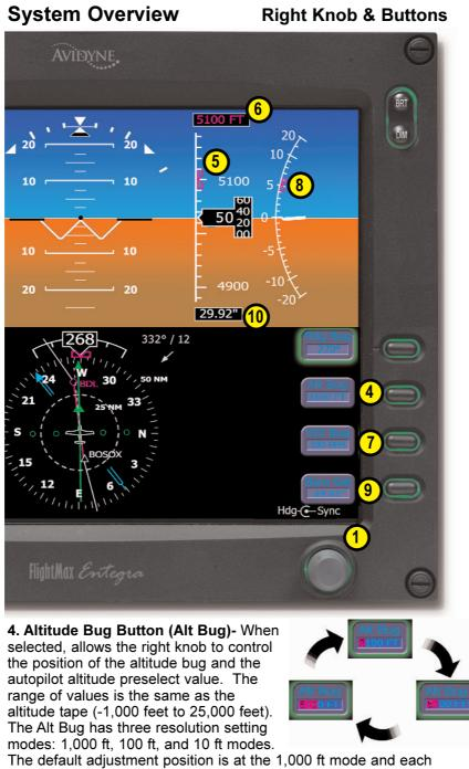
The default adjustment position is at the 1,000 ft mode and each button press steps the adjustment position down one place. The selected numeric value appears in the button and in the Altitude Preselect window.
