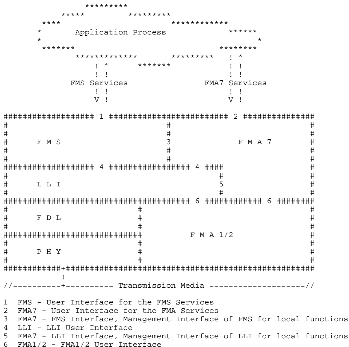
Figure 1. Placement of FMA7 in the ISO/OSI Layer Model
