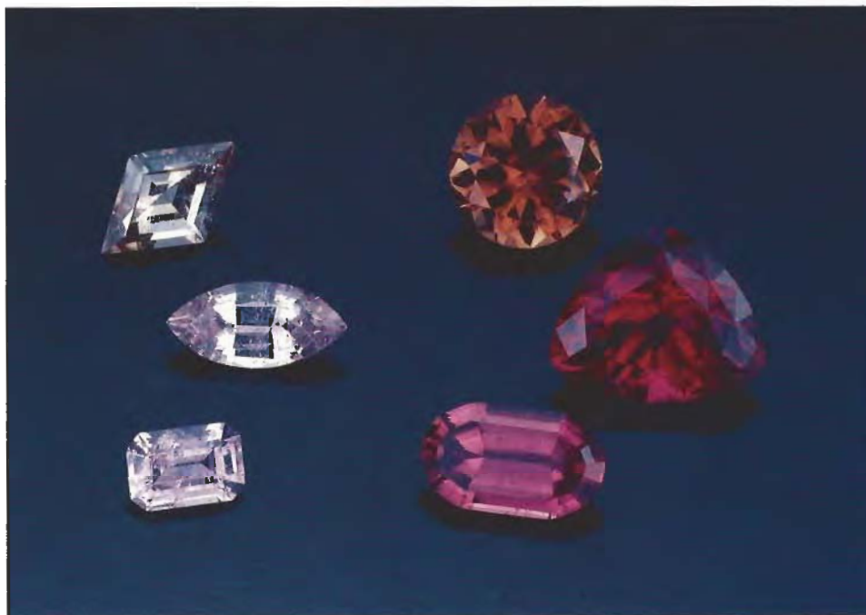
Figure 7. Today, pale colored tourmalines similar to those on the left are commonly irradiated with gamma rays to produce darker stones, like the irradiated tourmalines on the right (the largest is 5.91 ct). Stones courtesy of George Drake and the GIA collection; photo © Tino Hammid.
