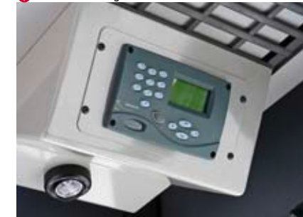
▼ Control unit for destination equipment with driver's light.
