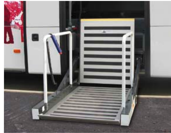
▲ Possibility for installation or preparation of wheel chair lift (with double doors, floor mounted fixation points and electrical wiring).
