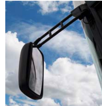
▲ Simple but functional rear view mirrors electrically heated (electrically controlled, as option).
