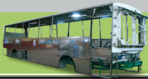
◀ Body structure with stainless steel panels
