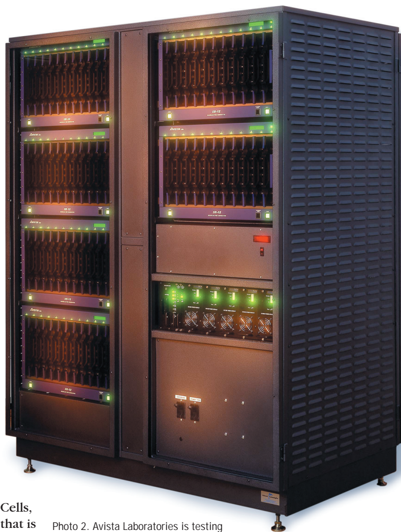
Photo 2. Avista Laboratories is testing prototypes of its residential fuel cell power system.
