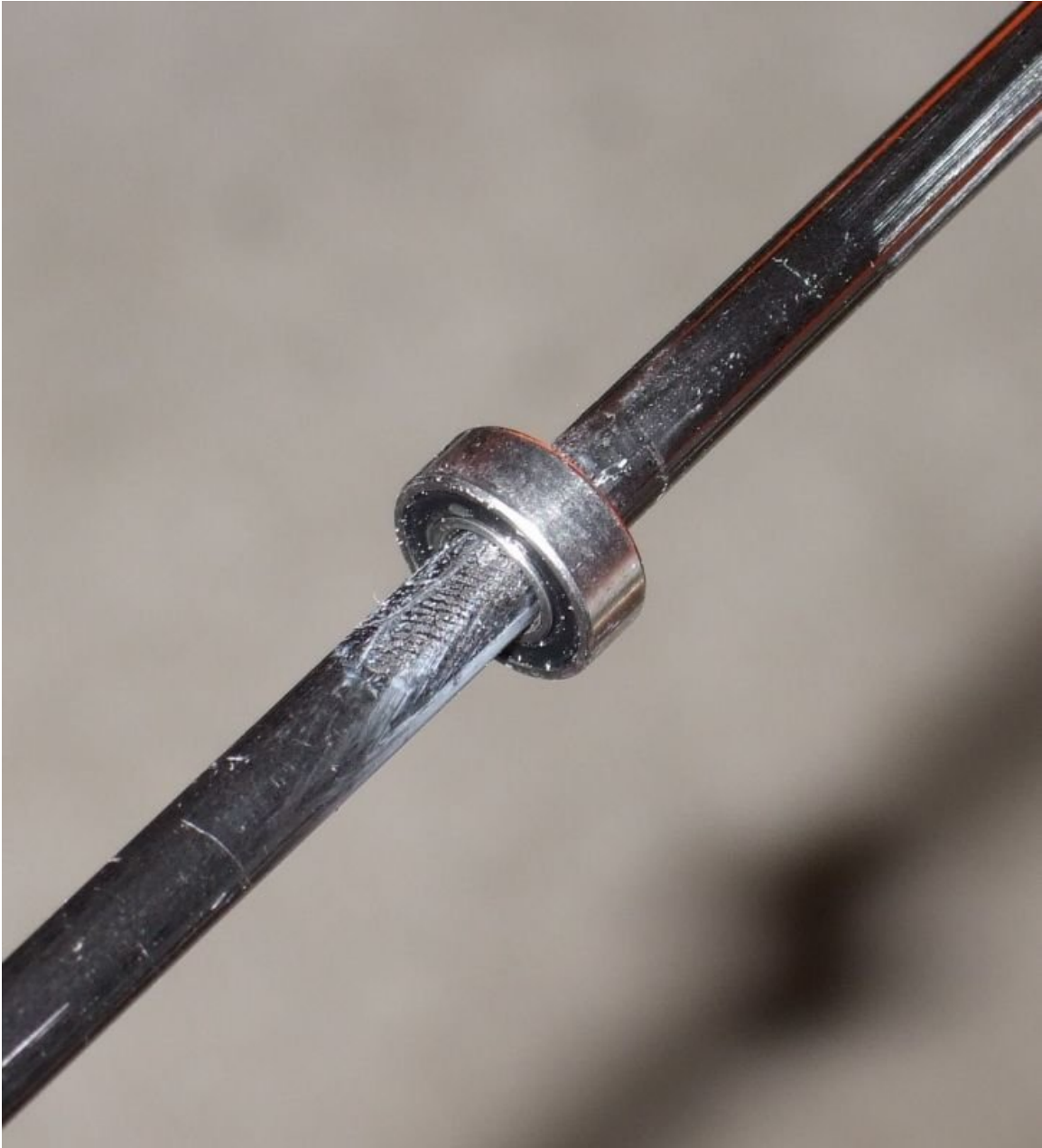
Rear end of prop shaft with guide bearing
