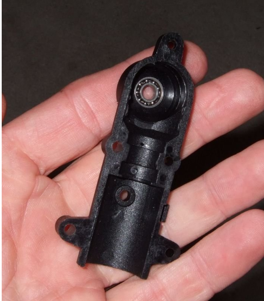
One Half of gear box with 5x11x4 bearing inserted
