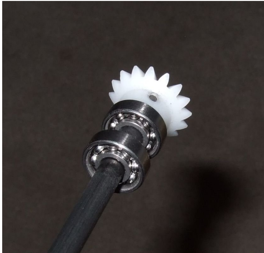
Front end of Prop-Shaft with two 5x13x4 bearings and large bevel gear
