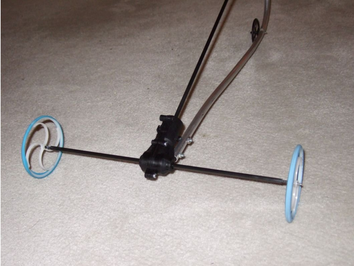
Front end – showing axle, wheels, prop-shaft, gear-box, and aluminum “frame”
