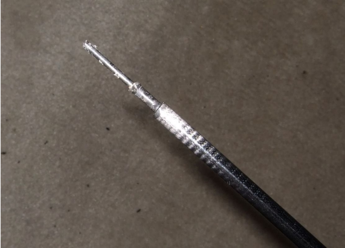
End of front axle with “step down’s”
