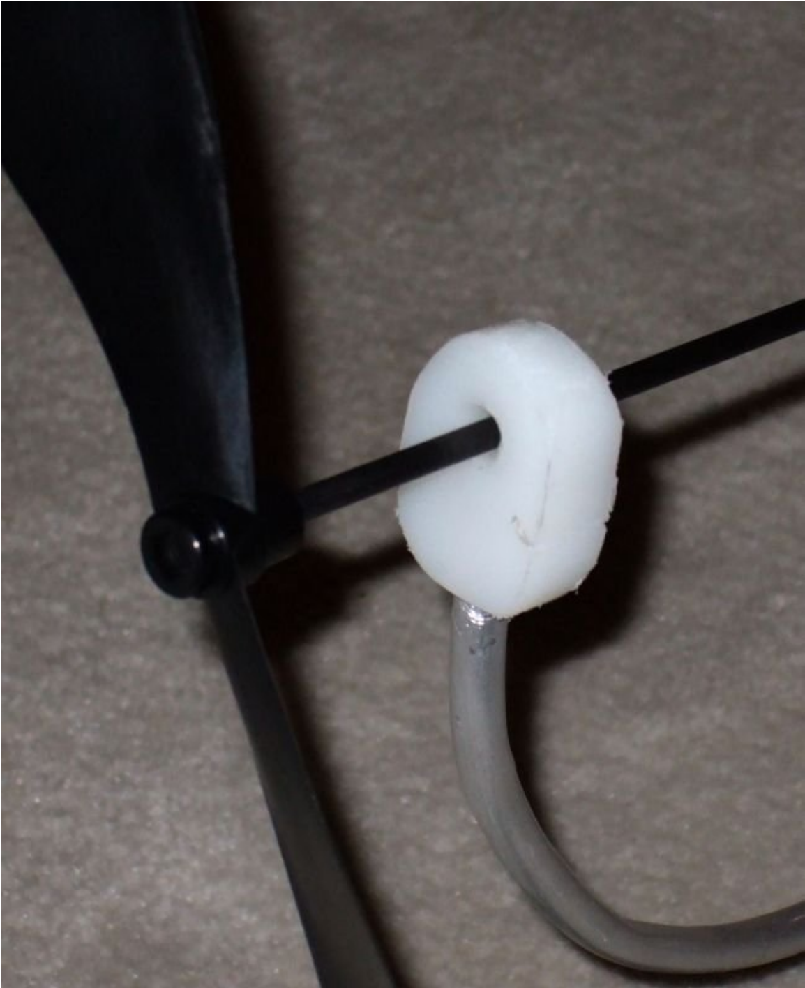
Tail end – showing aluminum “frame” going into HDPE bearing block
