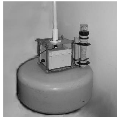
Figure 3. Photo of prototype buoy with attached radio/kOS enclosure.
