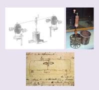
Extract from Joule's notebook showing the paddlewheel experiment demonstrating that mechanical energy causes friction and a rise in water temperature.
