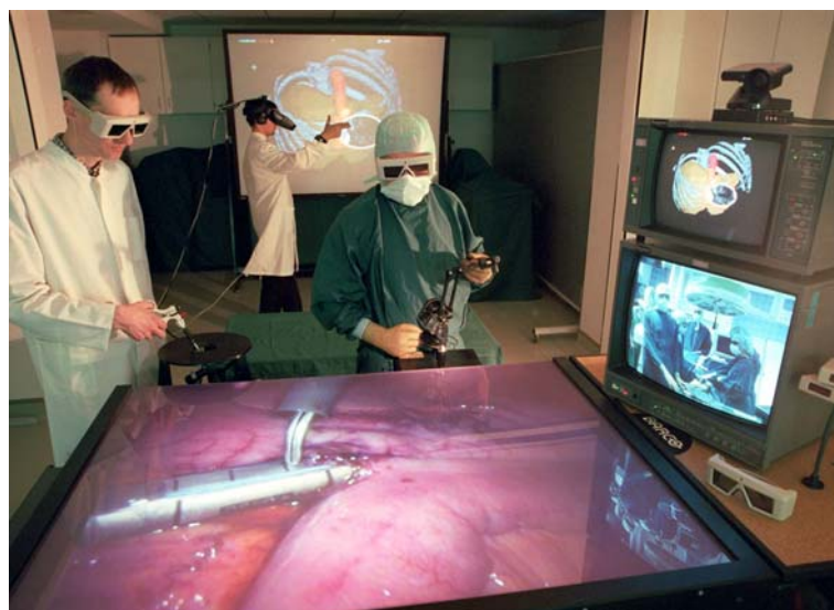
Fig. 1. Surgical Table for operation planning, simulation and training of surgical procedures. Two users can simultaneously observe tracked, stereoscopic views of virtual objects and work interactively (Integration of haptic feedback is in progress).
