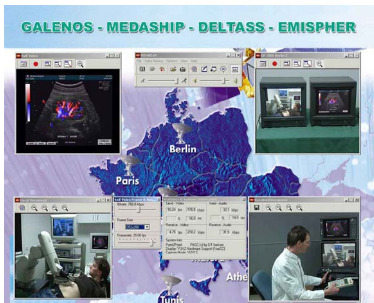
Fig. 2. MEDASHIP telesonography demonstrator. The expert (bottom right) can diagnose the patient (bottom left) from the US-images transmitted in real-time (top left). The expert can also remotely control the ultrasound (US) head (bottom left) (work in progress).
