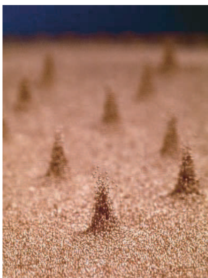
FIGURE 137 Oscillons formed by shaken bronze balls; horizontal size is about 2 cm (© Paul Umbanhowar)
