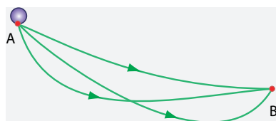
FIGURE 91 What shape of rail allows the black stone to glide most rapidly from point A to the lower point B?
