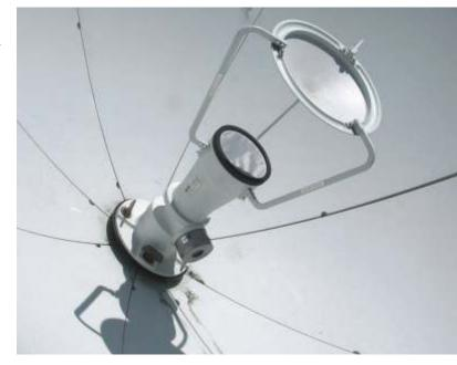
The antenna-mounted electronics enable the modem group to be located up to 50 metres from the selected antenna. Only three lightweight cables are required for the cross-site link for transmit, receive and control. Two high capacity modems can be used, as can ECCM types.
