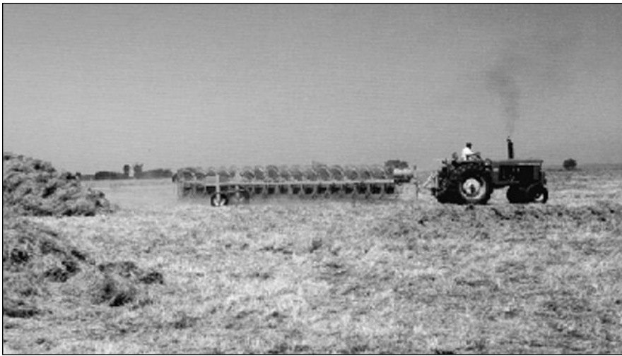
Figure 2. — Using a ground-driven wheel rake to clear a field of its full straw load.
