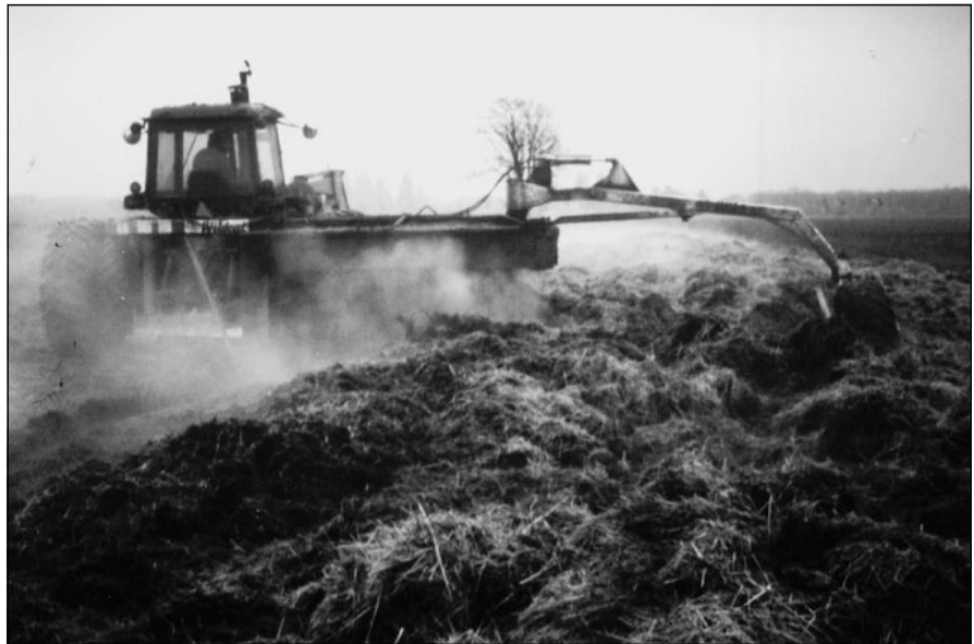
Figure 1.—Turning a grass straw windrow using a tractor-mounted compost turner.
