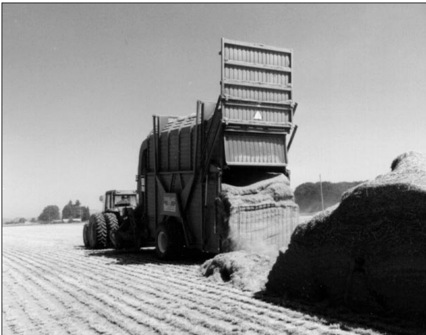
Figure 5.—Forming a short straw windrow with a flail-vac and stack wagon.
