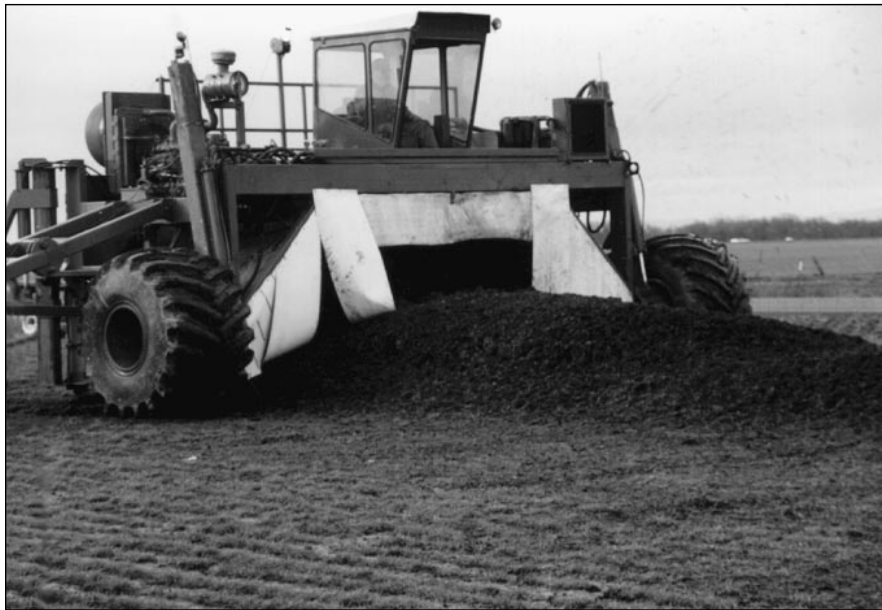
Figure 6. — Using a straddle-type compost turner on a short-straw windrow that is composting.
