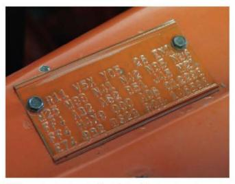
With its prominent location on the driver's fender, the fender tag is usually easy to locate. 1965 and earlier cars may have it on one of the following locations: left inner fender, right inner fender, right cowl panel, left radiator core support.
